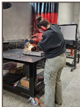
Emily preparing the rebar by cutting it down to size with a chop saw
