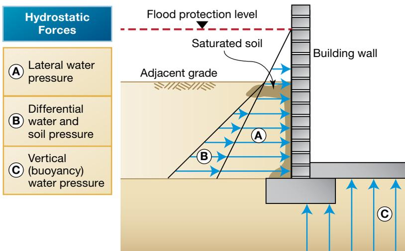
Figure 3-4. Hydrostatic loads
