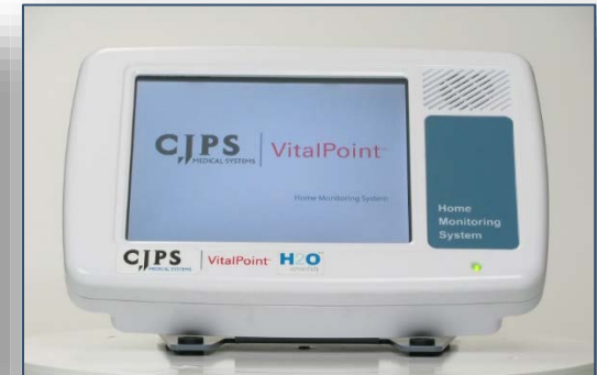
A home patient monitor that measures blood pressure, pulse rate, blood oxygen saturation, weight, glucose level, prothrombin time, fluid status and temperature. Image: 4mdmedical.com
