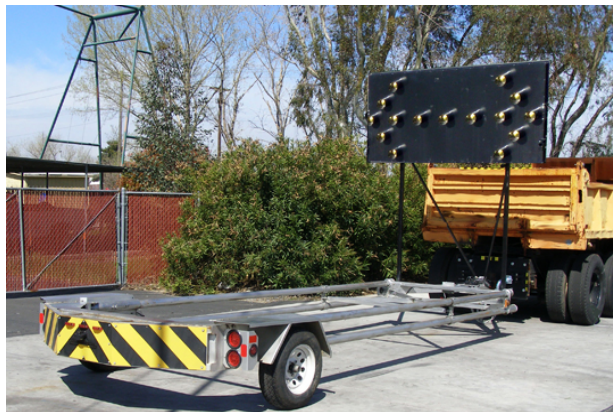
Impact attenuator trailer with arrow board
