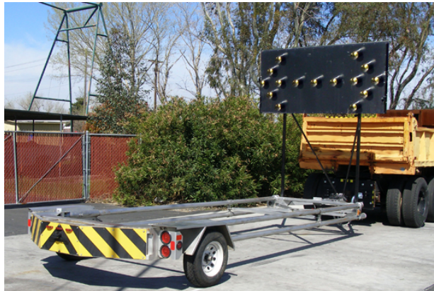
Impact attenuator trailer with arrow board
