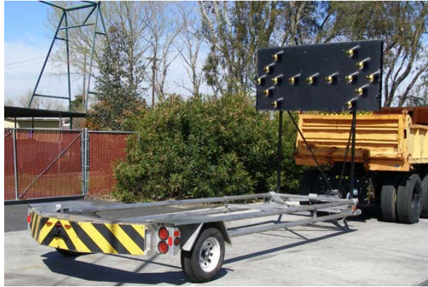
Impact attenuator trailer with arrow board
