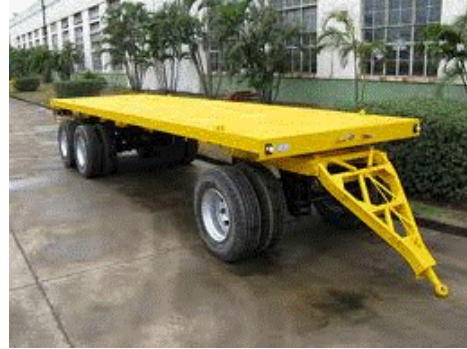
Semitrailer (part of the weight rests on the pulling unit) Full-trailer (weight does not rest on the pulling unit)
