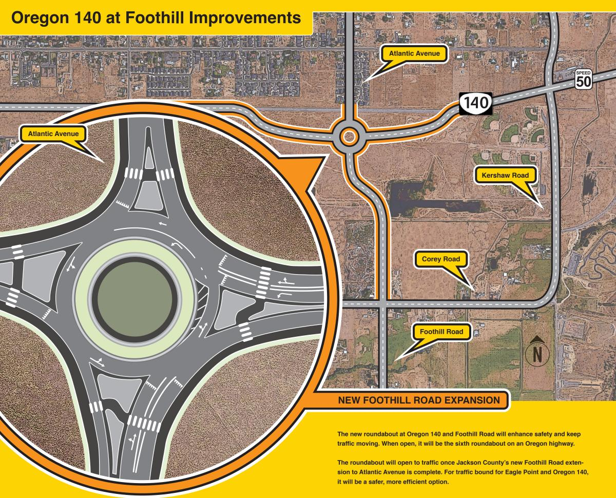
For safety, the existing Kershaw Road intersection will be changed to eliminate the highway crossing. Traffic will still be able to use the modified intersection for right in, right out and left in movements.
