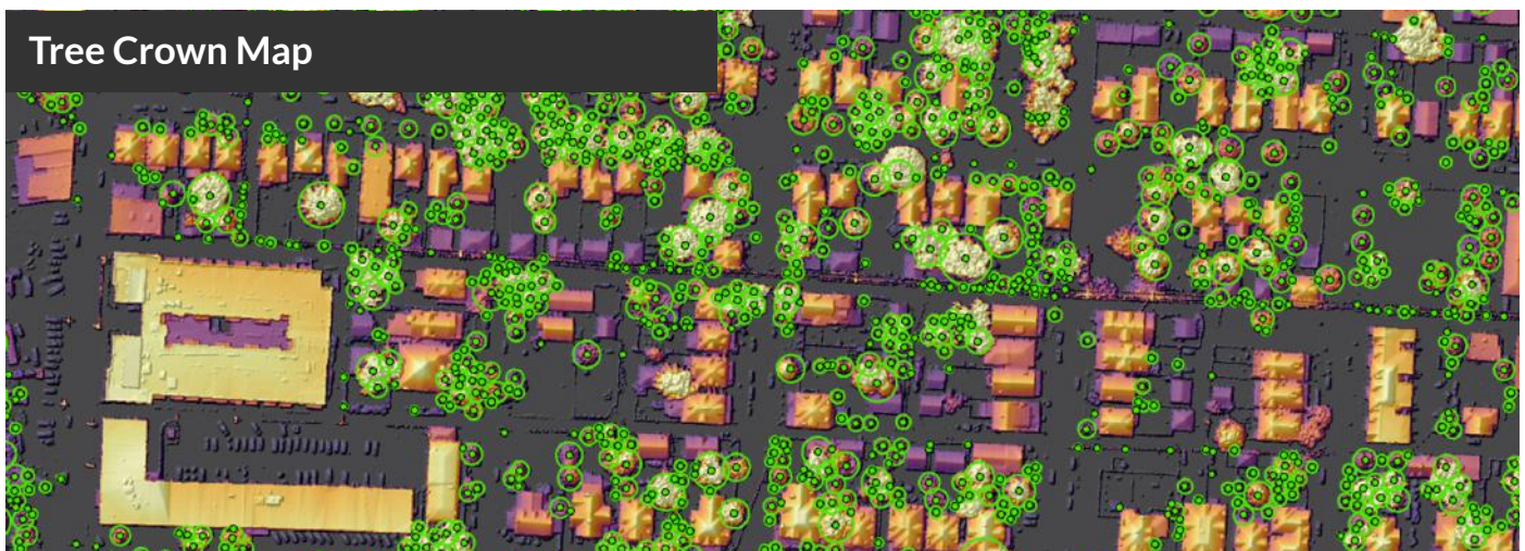
Figure 6: Tree centroids (dots) and tree crowns (circles) mapped from the 2019 LiDAR. Tree mapping from LiDAR involves finding relative high points for each tree, then tracing down until a height inflection point is reached, marking the edge of the crown. This approach to individual tree mapping is most accurate where there is a clear differentiation in tree crowns and is less accurate in forested stands where crowns may overlap.
