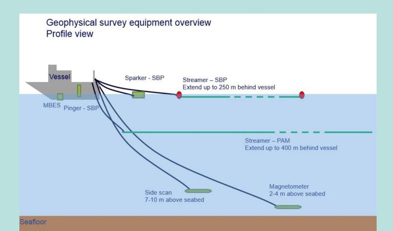
Above: Schematic diagram of proposed geophysical and marine mammal survey equipment towed behind the *R/V Enterprise*.
