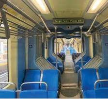
Metro Transit is installing more than 13,000 custom designed plastic seats on all 91 light rail vehicles. This follows testing plastic seats on a handful of vehicles last year. For the past 16 years, vehicles had cloth seats, which proved difficult to keep clean and dry, especially during winter months. The new Green Line Extension vehicles will also feature plastic seats. Customers are invited to offer feedback on the new seats by contacting Customer Relations.
