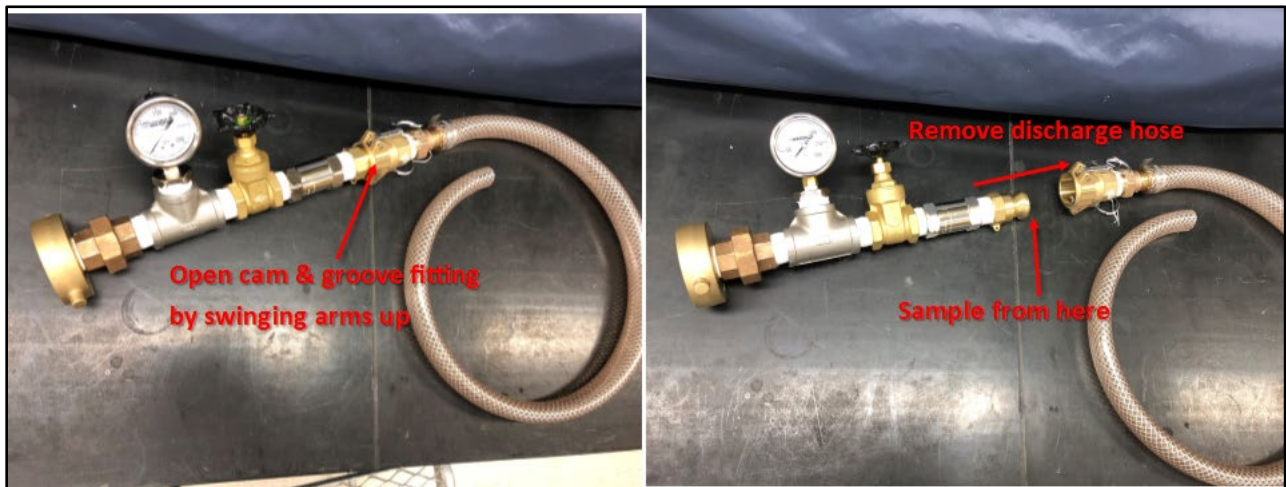
Figure 6. Removing discharge hose for sample collection
