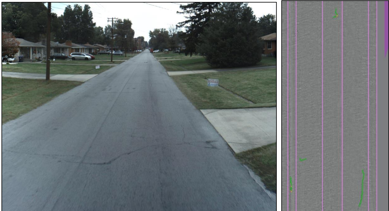
Figure 5.2.1.a : Mandli Right of way (ROW) imagery of a road with a PCI score of 87 , which is considered Good (Left). Figure 5.2.1.b: Image of the LCMS Rage Downward Image with Overlay of the road depicted in Figure 5.2.1.a.
