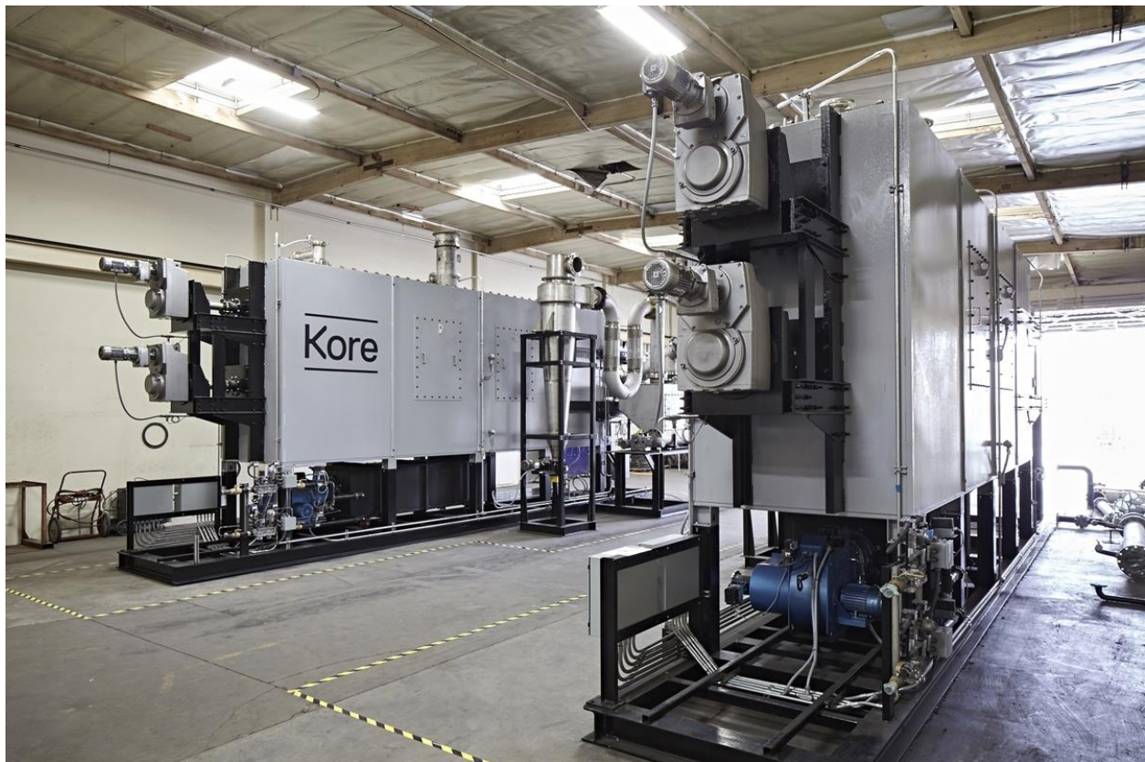
Kore Infrastructure's pyrolyzers, which are used to convert biomass into carbon-negative hydrogen, renewable natural gas and biogas. (Image courtesy of Kore Infrastructure.)
