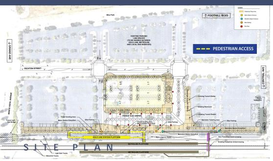
The Montclair Station will be located at the Montclair TransCenter, just east of Monte Vista Avenue and north of Arrow Highway. The A Line station will be a center platform station, with light rail tracks on either side (one for westbound and one for eastbound trains) and will be located to the north of the existing Metrolink platforms. A connection will be built between the A Line and Metrolink platforms via the existing pedestrian tunnel to facilitate pedestrian movement between systems.
