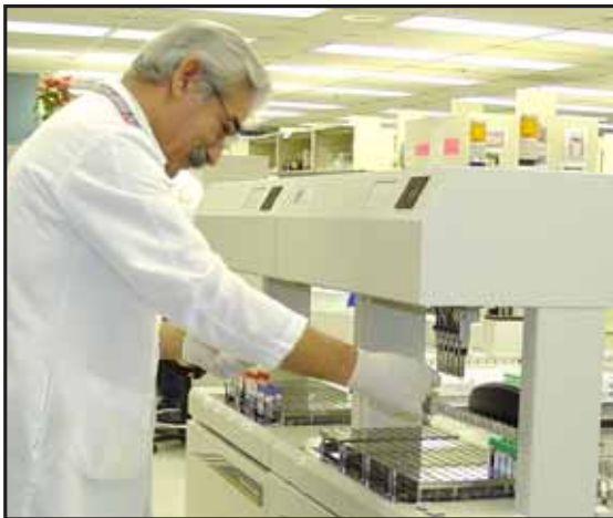
Supervisory Medical Technologist Ramiro Garza sorts samples into the robotic processor racks. The robotic processor runs up to 600 tests per hour and includes such safety and quality-control features as cap piercing, "flags" when irregularities appear or results are outside normal ranges, automatic creation of slides when abnormalities are detected, and automatic dot detection.
