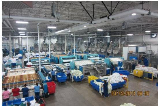
HSCL production floor with automatic gas dryers using energy-efficient venting systems to capture and transfer exhausting heat to incoming fresh air.
