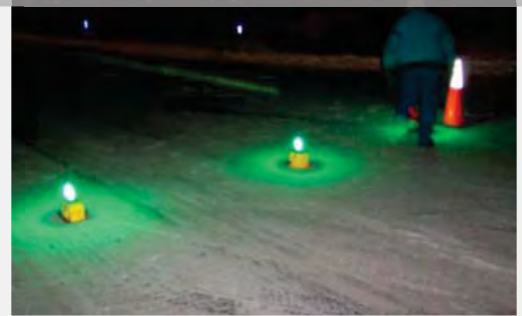
Top –DLG’s new runway lights trailer fits into smaller aircraft that serve rural airports. Bottom - on a clear night emergency lights are visible 5 miles out on approach to the airport.
